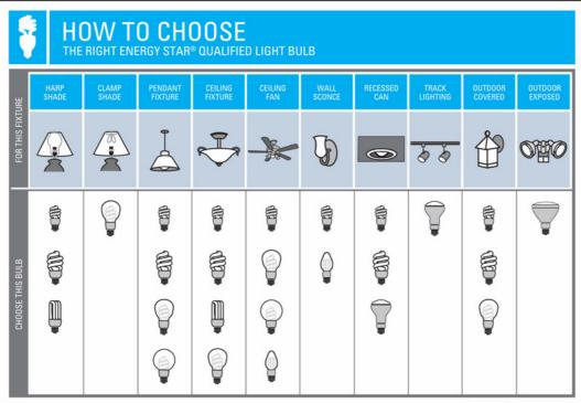
NOTE: If your fixture is connected to a dimmer or three-way switch, do not place an ENERGY STAR qualified light bulb in the fixture unless it is labeled as appropriate for dimmers or three-way switches.
